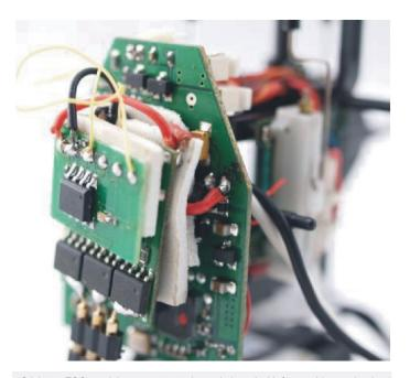
Stick two ESCs and the converter to the main board with foam rubber under the circumstance of correct circuit connection.
