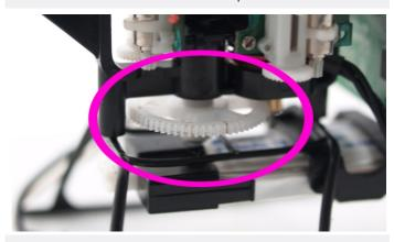
4. Assemble main gear and prop, make sure the right position of main gear and pinion gear.
