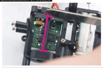
1. Separate the linear servo, then cut the support column on the frame and make it smooth.
