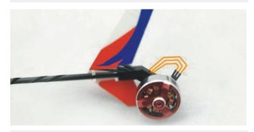
5.Insert the tail brushless motor into the matched hole position, get the wire from one side through the tail tube to another side, then connected it to tail motor ESC.
