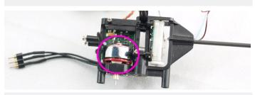
2. Assemble the pinion gear to the main brushless motor then assemble it into the frame.
