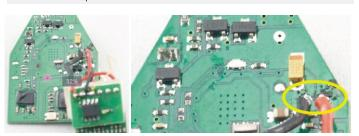
Converter gets power from main board side B (as picture shows) Voltage: 5V
