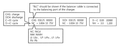
If the Enter button is pressed, the charge or discharge can be terminated.
