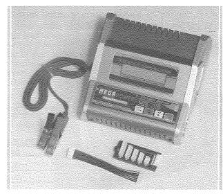
The set contains the MEGA POWER POSEIDON-860DS with a separate Thunder Power/Flight Power Type adapter board
